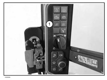
The lights button (Item 1) [Figure 33] is located on the right control panel.
