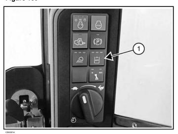
1. Press the auxiliary hydraulics button (Item 1) [Figure 139] on the right control panel once to activate auxiliary hydraulics.
