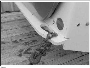
Install chains at both rear tie-down positions [Figure 209]. (Right side shown.)
