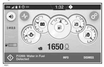
A notification [Figure 169] can alert you to a machine condition requiring service.
