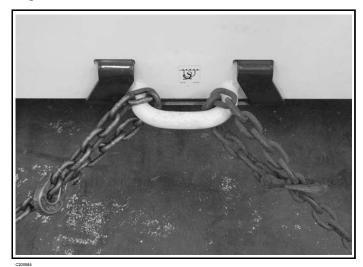
5. Install chains at the front tie-down position [Figure 210]. (Lift arms shown raised for visual clarity.)
