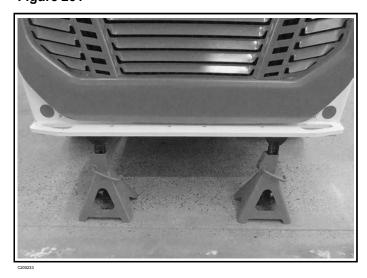
3. Install jackstands under the rear of the machine frame [Figure 231].
