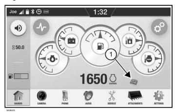
The service schedule information is based off the machine service schedule. The display will notify the operator 10 hours prior to the next service due and continue until the service is completed (Item 1) [Figure 389].
