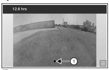
Ensure the camera is centred left and right. The mark on the ground (Item 2) [Figure 29] from step 1 should be visible on the display. Continue with procedure if necessary.
