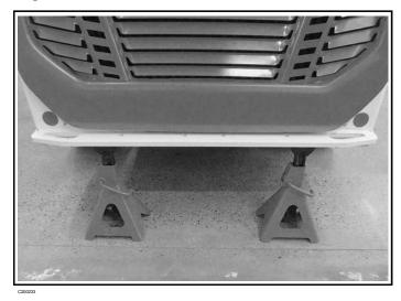
2. Put jackstands under the rear of the machine frame [Figure 222].
