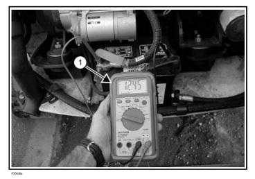
The simplest and most common check to determine battery state of charge is to use a digital multimeter or voltmeter (Item 1) [Figure 292].
