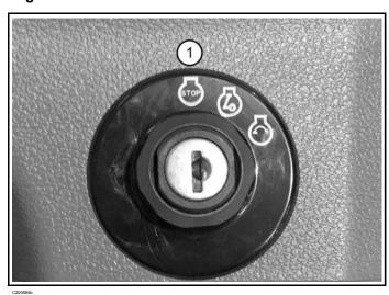
Press the stop button (Item 1) [Figure 170] or turn the key switch (if equipped) to the Stop position (Item 1) [Figure 171] to stop the engine and turn the machine's electrical system OFF.
