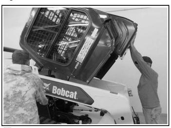
Pull down on the bottom of the operator cab until stopped by the latching mechanism [Figure 234].
