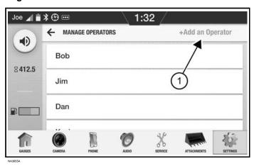
Select [ADD AN OPERATOR] (Item 1) [Figure 436] to enter a new operator.
