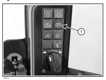
Press the parking brake button (Item 1) [Figure 62] on the right control panel to engage the parking brake.
