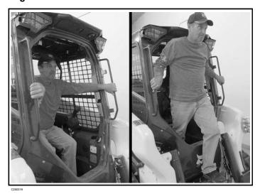
Exit the machine using grab handles, safety tread, and steps (maintaining a three-point contact) [Figure 172].
