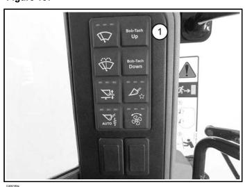
Push and hold Bob-Tach Wedges Up button (Item 1) [Figure 187] on the left control panel until levers are fully raised (wedges fully raised).
