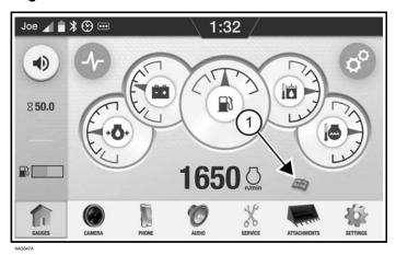
The service schedule information is based off the machine service schedule. The display will notify the operator 10 hours prior to the next service due and continue until the service is completed (Item 1) [Figure 394].
