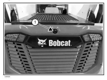
The rear view camera (Item 1) [Figure 28] is located in the rear door.
