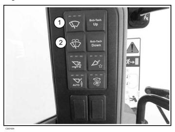
If equipped with front wiper and washer, the controls (Items 1 and 2) [Figure 34] are located on the left control panel.
