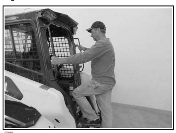
Use the bucket or attachment steps, grab handles, and safety treads (on the machine lift arms and frame) to get on and off the machine, maintaining a three-point contact at all times [Figure 147]. Do not
