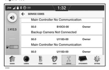
Scroll down to see a history that shows the machine hours, the date, and the operator logged in each time the code was activated [Figure 407].
