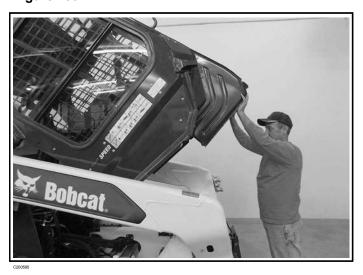
Push the bottom of the operator cab [Figure 233] slowly until the operator cab is all the way up and the latching mechanism engages.
