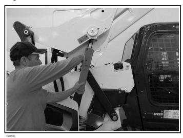
Have a second person install the lift arm support over the rod of one of the lift cylinders [Figure 224].
