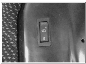
The switch [Figure 153] to turn the heated seat on or off is located behind the seat back on the left side.
